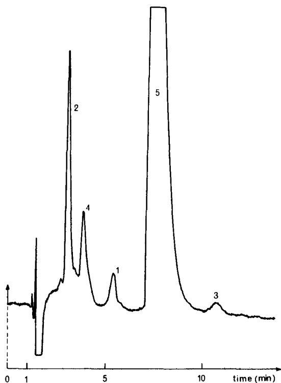
Fig. 3. Analysis of a TOPO A sample. Column: LiChrosorb RP-8, 5 \mu\text{m} , 10 cm \times 4.6 mm I.D. Mobile phase: methanol-phosphate buffer pH 7.5-methylene chloride (85:15:9) + TDA bromide (0.15 g per 100 ml). Peaks as in Fig. 2.
