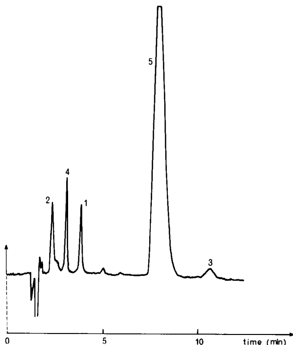
Fig. 2. Analysis of a TOPO B sample. Column: Hypersil C_8 , 5 \mu\text{m} , 10 \text{ cm} \times 4.6 \text{ mm} I.D. Mobile phase: methanol-phosphate buffer pH 8-methylene chloride (85:14:9) + TOA bromide (0.3 g per 100 ml). Peaks: 1 = A1 acid; 2 = A2 acid; 3 = phosphinate; 4 = DOPO; 5 = TOPO.
